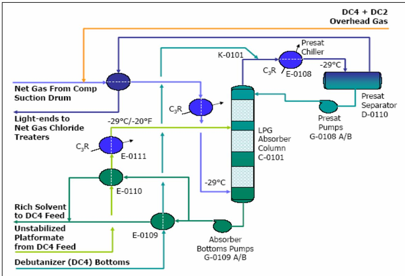
**Figure 2 - LPG Absorber Configuration at Yanbu' Refinery**
