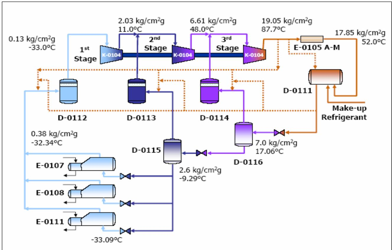
**Figure 4** – Three-Stage Propane Refrigeration Cycle for LPG Recovery
