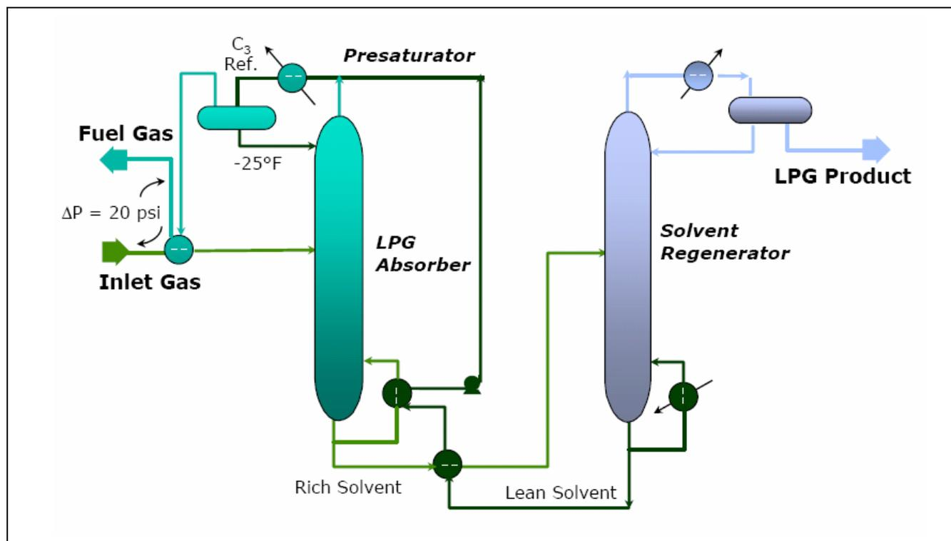
Figure 1 - AET Process LPG Recovery Unit <sup>1</sup>
